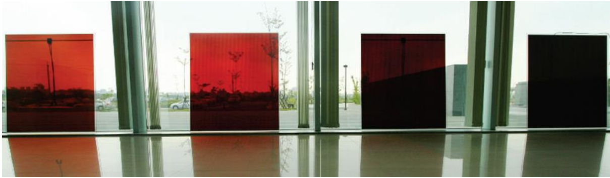
Fig.8: Module BIPV transparente cu STHSC de diferite grosimi, fără straturi reflectătoare STHSC see-through BIPV modules of different film thicknesses and without the reflective layers
